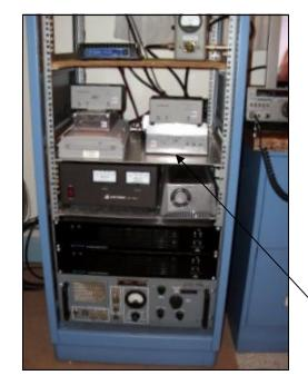
The rack all wired up and in place. The bottom is the AM-6155 amp. Above that are 2 – GlenAyre 28v 25amp power supplies. Above that on left is an Astron RS35M 13.8v 25amp supply. On right is a Power Source 13.8v 75amp switching power supply. Above that is 903 & 222 transverters with sequencers and power amps. Above that is a Teletec 432 amp that puts out 150 watts.
