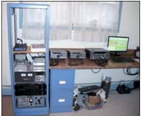
Front view of station. Equipment rack, Kenwood TS-430s for 903, Kenwood TS-430s for 222, Yaesu FT-736R from Bill, K3EGE, for the January contest. My 20" LED Monitor screen, wireless keyboard and mouse. The new PC under the counter is an HP Pavillion Slimline with 6 G memory and a 1 Terabyte hard drive. It has a UPS System in case of power failure to safely close down the system.
